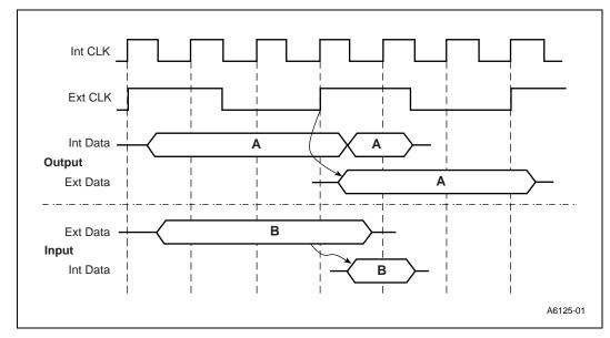
Figure 16-19. Processor 1/3 Bus Internal/External Data Movement
